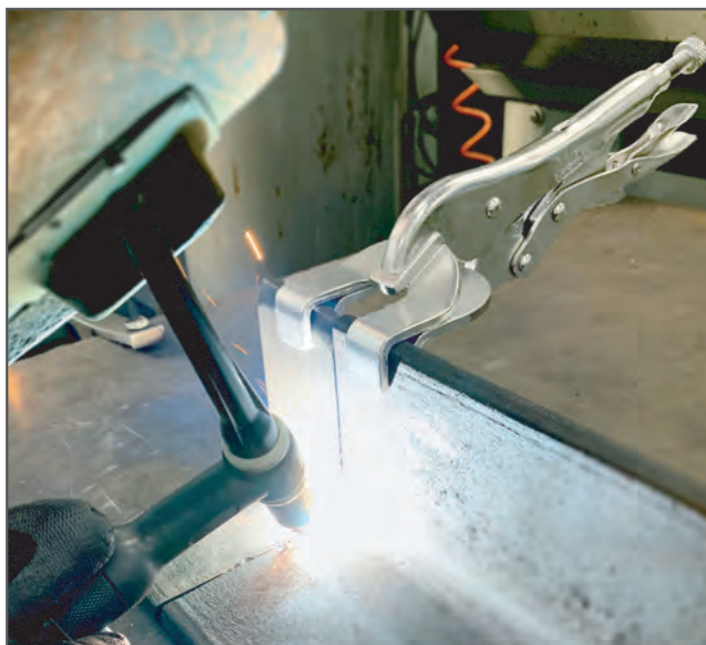
Bottom jaw slides in a straight-line motion to hold penal in place when locking.
