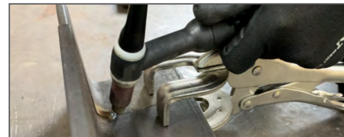
The over-reaching split upper jaw let you clamp pieces in place and still have room to weld or at least firmly tack them in place for full welding later.
