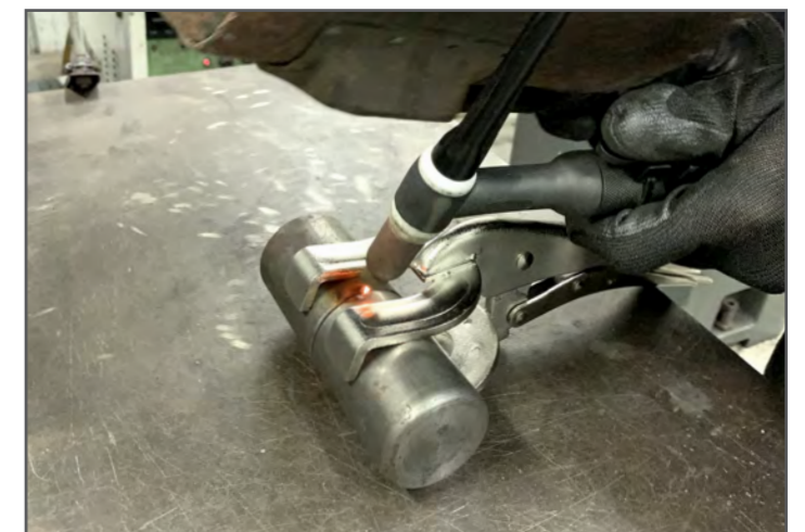
The over-reaching split upper jaw let you clamp pieces in place and still have room to weld or at least firmly tack them in place for full welding later.
